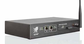
The Multichannel VPN Router 200 was designed especially for use in home offices and while travelling. With this device, an existing Internet connection can be bonded with another one — by that, the achievable bandwidth and reliability can be enhanced at very reasonable costs by combining a landline medium like DSL or cable with a mobile data connection like UMTS / 3G or LTE / 4G.
